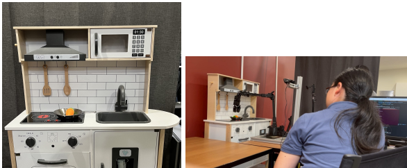
Figure 9. (Left) Closeup view of the kitchen set with the spoon hanging on the wall, above the pan on the stove. (Right) For the experiment: WidowX 250 6DOF robot arm, user, and desktop to input user feedback.
